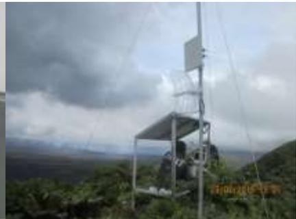
*The technician is checking the transmission quality of the Air Grid at MANTOWER RELAY (AMCR)*
